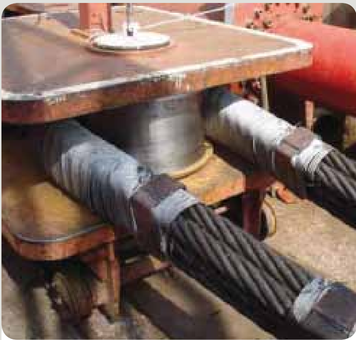
Testing of a KimFlex Sling showing the eye construction.
