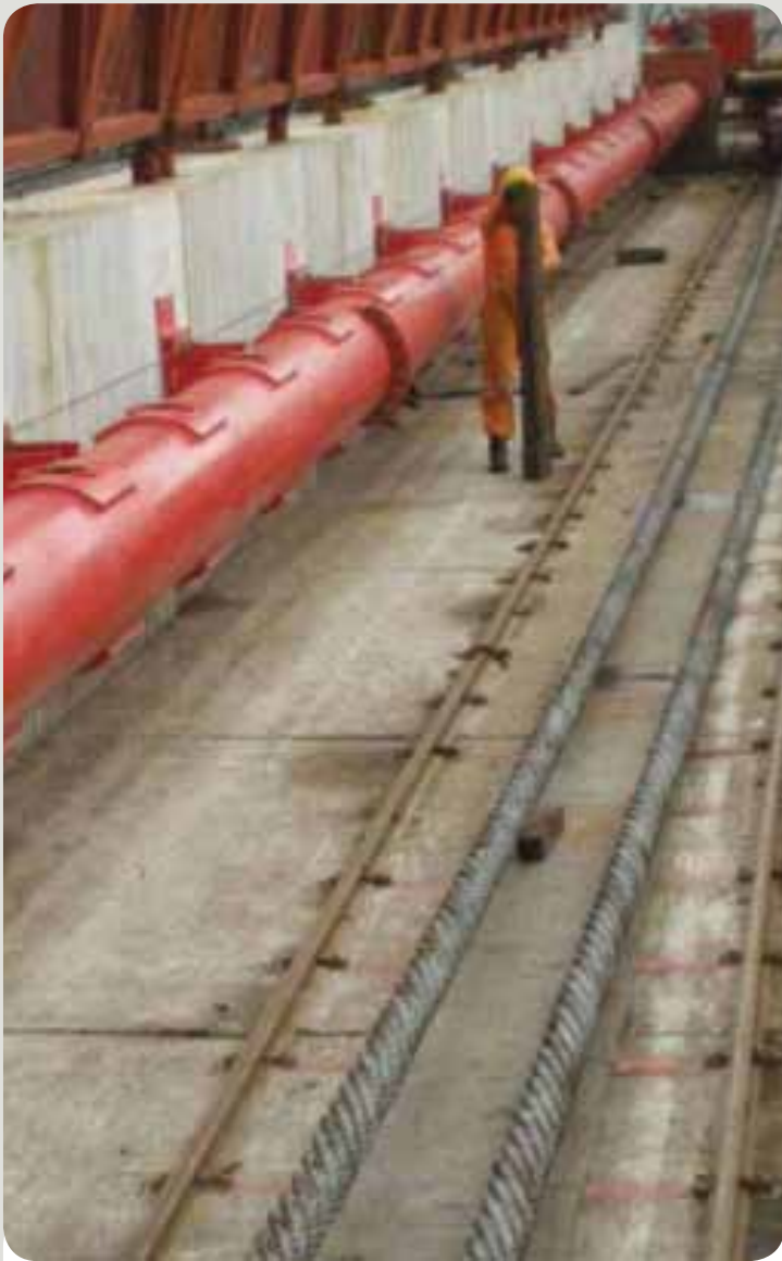
Testing of a 20 m long Cable Laid Grommet.
