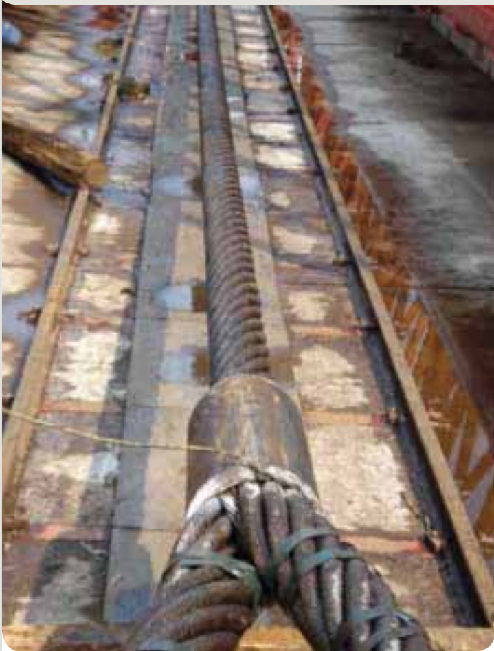
Testing of 6” dia KimSwage Sling.
