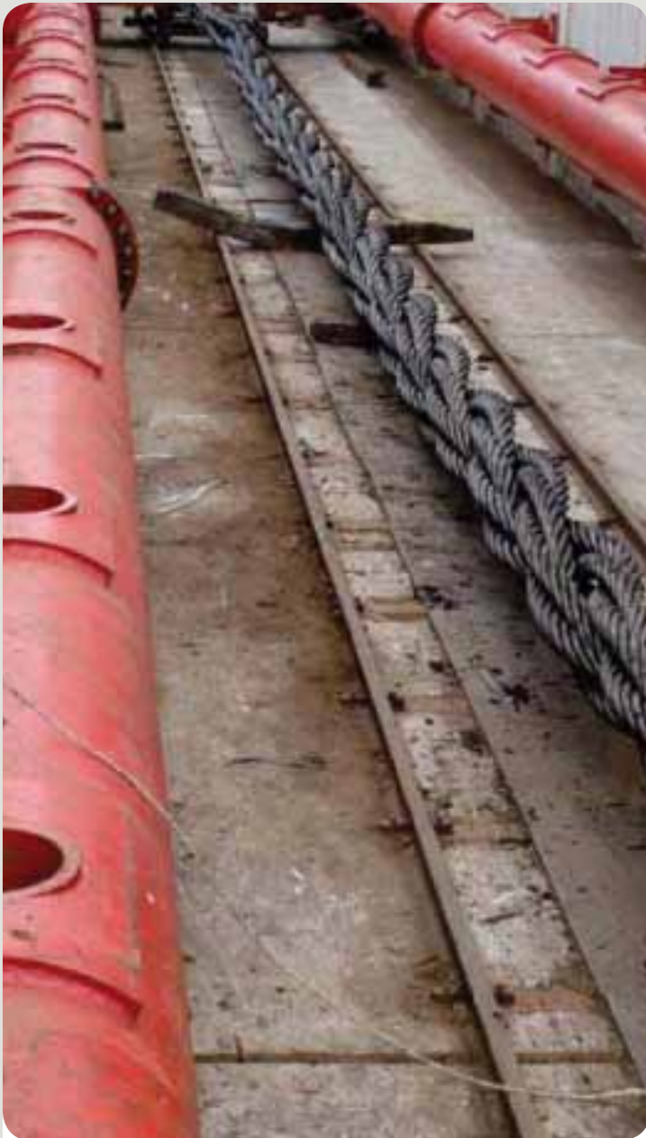
Proof load testing of a KimFlex 9" dia Sling in KimTest 3000 test bed to the client's strict length tolerance.
