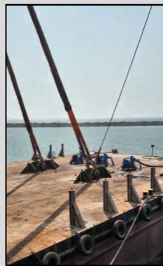
The KLX-815 slings had been used for multiple offshore heavy lift projects, including lifting top decks and load testing (shown above)
