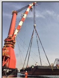
The KLX-815 slings had been used for multiple offshore heavy lift projects, including lifting top decks and load testing (shown above)
